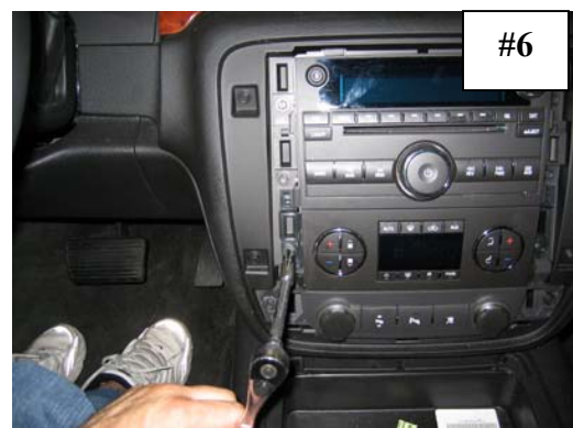
Remove factory trim screws to remove the lower switch panel on dashboard
